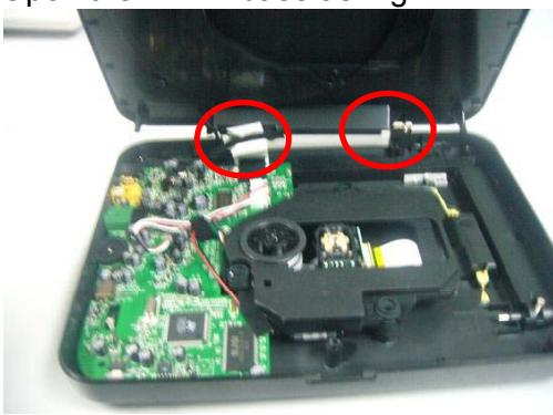
5.0 Remove screws to remove TFT PCB
